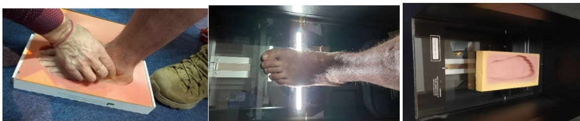
Figure 2: Obtaining information about the foot using the 3D scanner InFoot3D, creating a footprint on a polymer foam, and then scanning this polymer foam footprint
