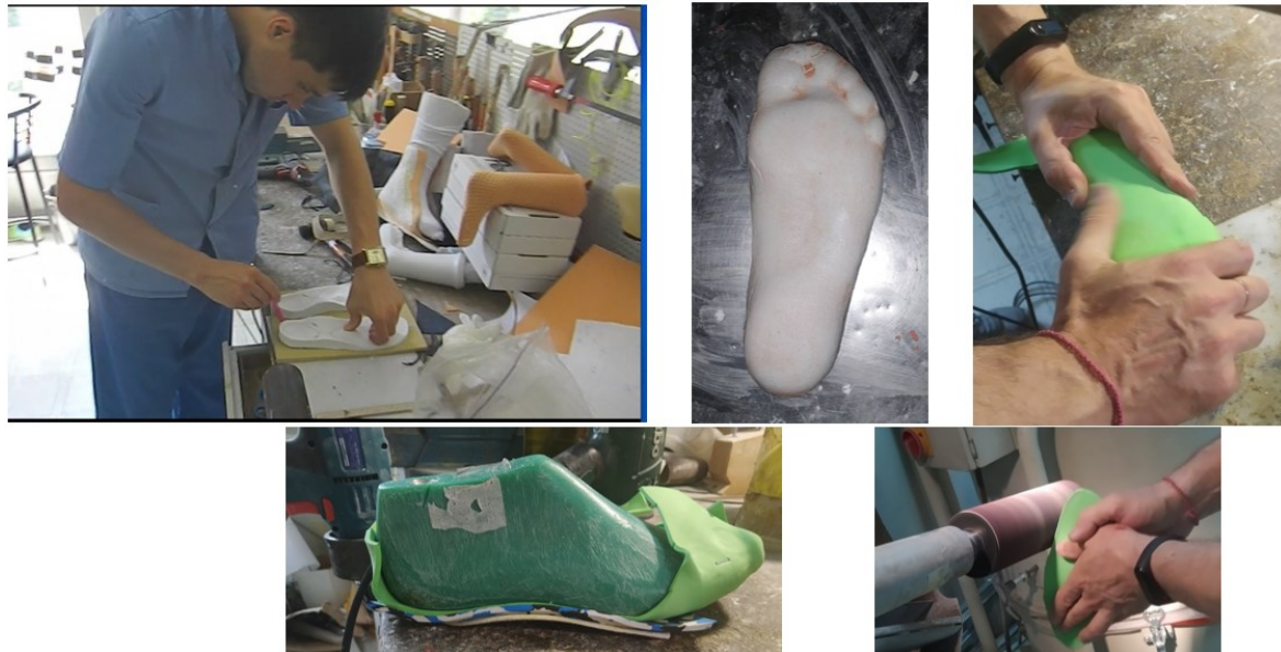
Figure 4: Classical method of making individual insoles to prevent of deformities of the foot
