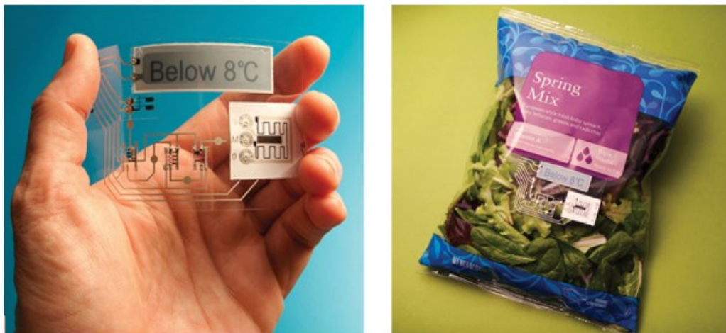
Figure 3: Intelligent packaging: a) example of external indicator, b) example of intelligent packaging
