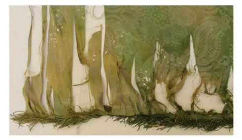
Figure 5. The very brittle state of a damask fabric as a consequence of low humidity
