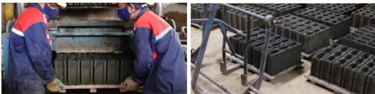
*Bricks created by mixing the sludge, the toxic waste of the denim process*
