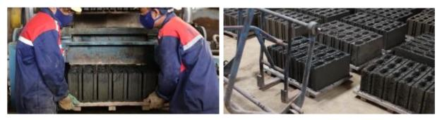
Bricks created by mixing the sludge, the toxic waste of the denim process
