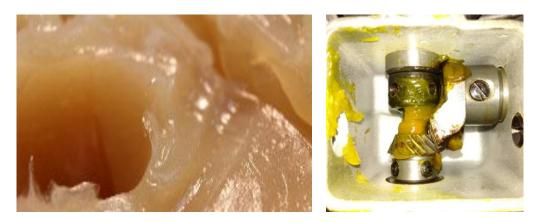
Figure 1. Grease (a) sewing machine parts lubricated with the grease (b)
