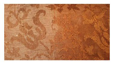
Figure 6: Discoloration of cotton fabric due to photo-oxidation
