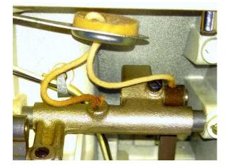
Figure 2. Felt oil pad and cotton wicks to distribute the oil
