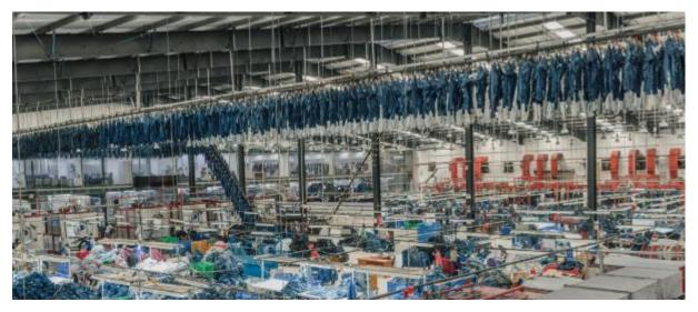
Air drying method for the denim products using air recycled from hot factory machinery
