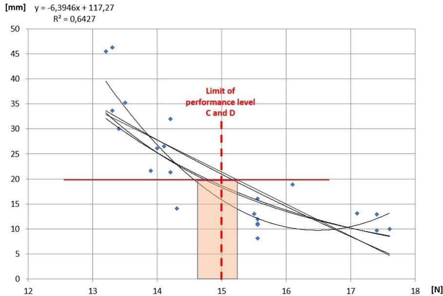
Figure 5: Differences in obtained cutting force values at a 20 mm cutting stroke length (curves of approximations with linear, quadratic polynomial, logarithmic, exponential and power functions) by selecting different regression curves for a typical TDM test result data set
