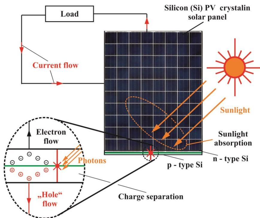
Figure 5: Working method of PV solar panel
