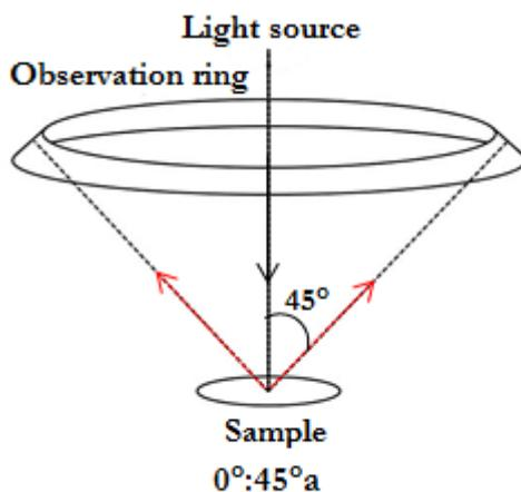
Figure 4: Directional geometry  $0^\circ:45^\circ a$
