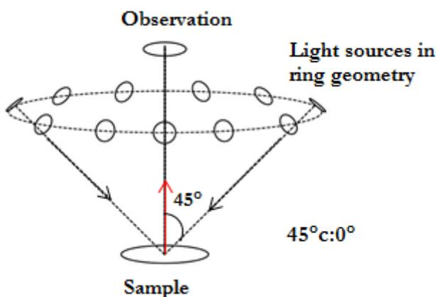
Figure 3: Directional geometry  $45^\circ c:0^\circ$
