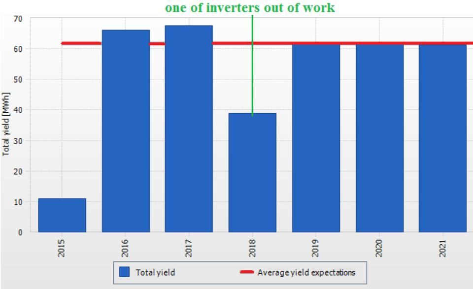
Figure 10: Total yield of the power station from 2015 to 2021 in MWh
