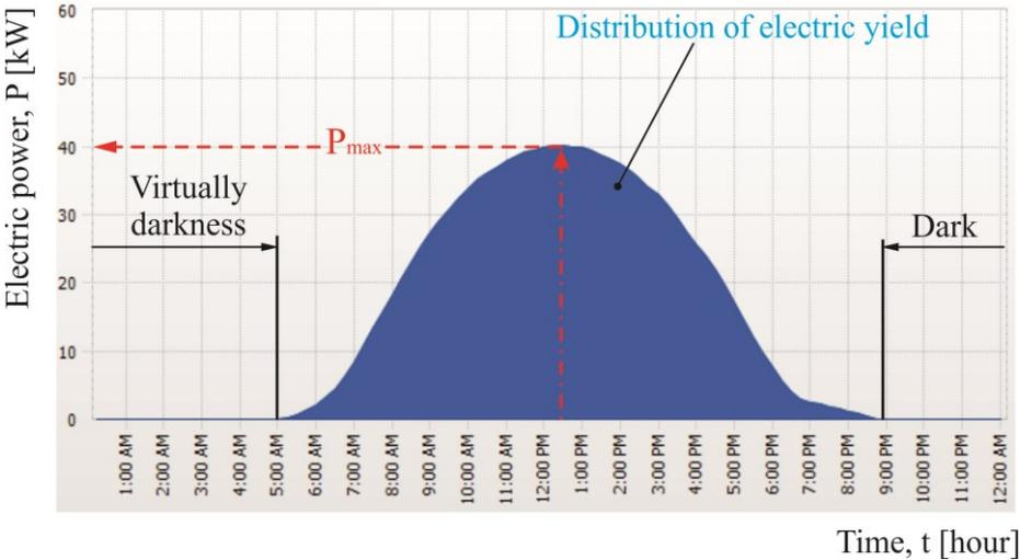
Figure 8: The distribution of the delivered power on the 15<sup>th</sup> of June, 2021 in kW
