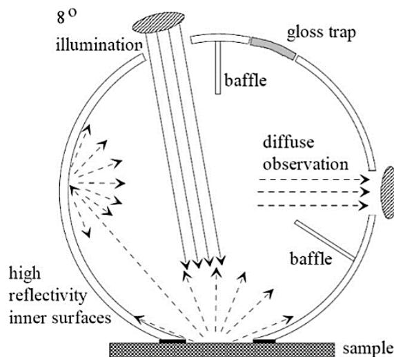
Figure 6: Measurement geometry  $de:8^\circ$
