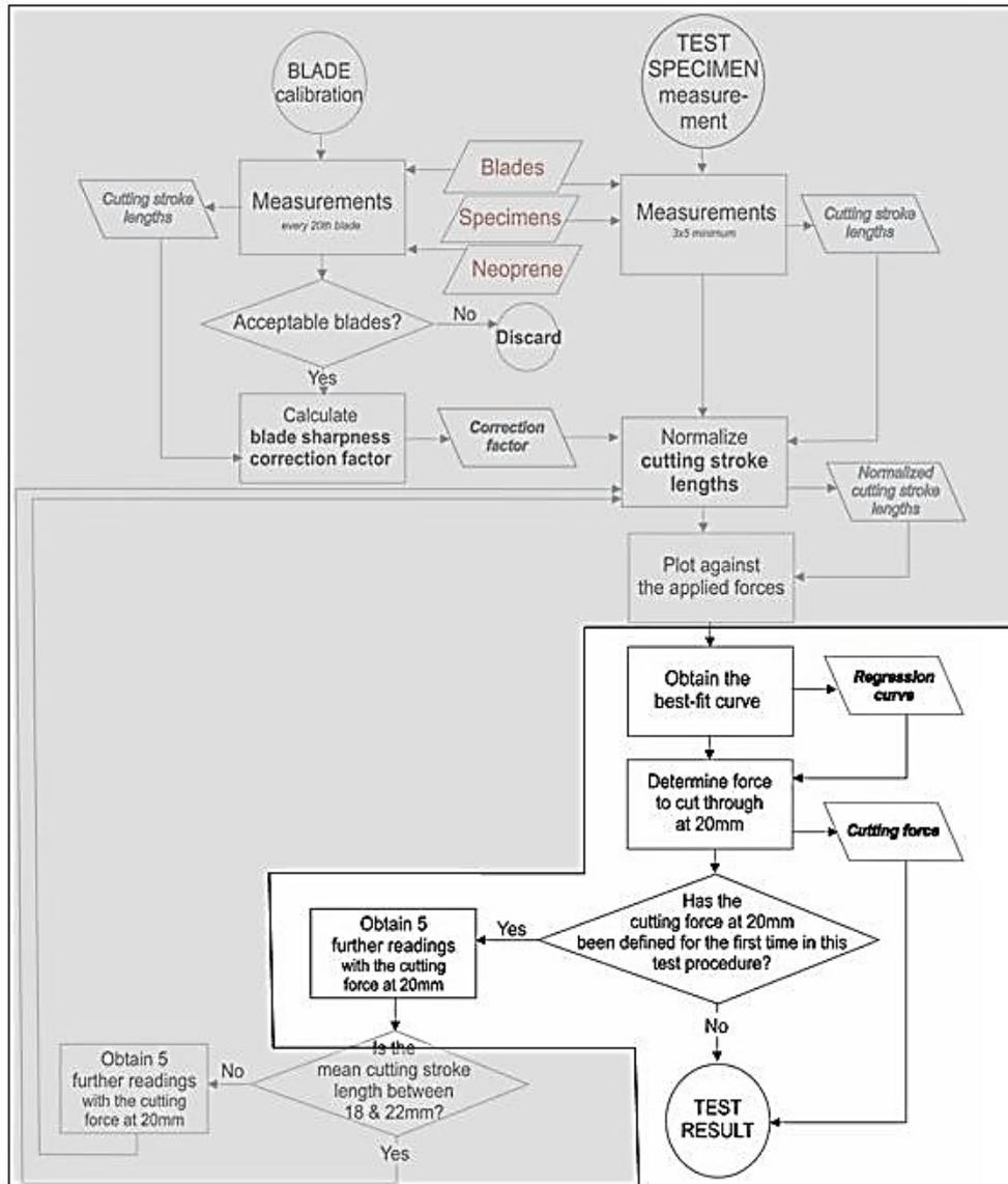
Figure 2: Test procedure according to ISO 13997:1999. The part targeted by this article is on white background [4]
