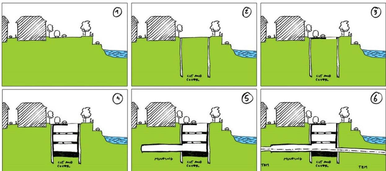
Figure 3: Steps for the metro's construction
