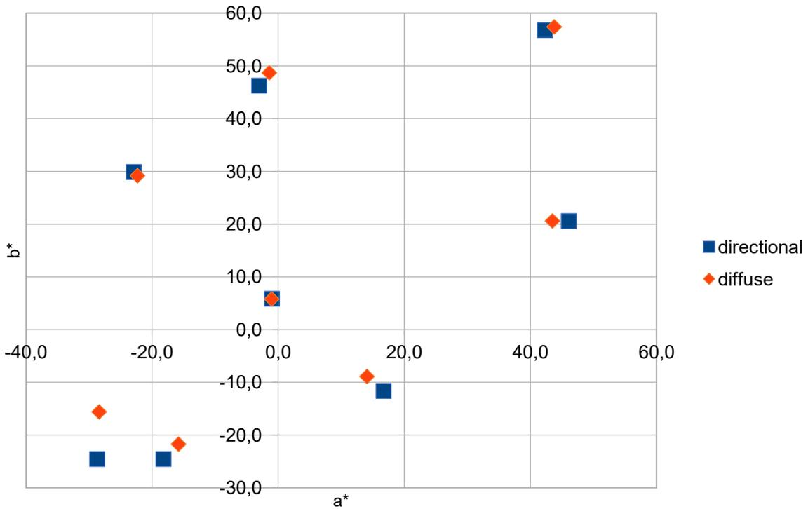
Figure 13: CIELAB  $a^*$ ,  $b^*$  values of the eight color samples with texture #4 on the chromaticity plane, obtained by instrument with directional (blue squares) and diffuse (orange diamonds) measurement geometry
