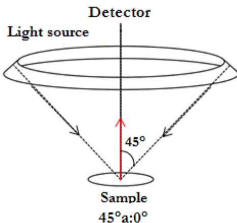
Figure 2: Directional geometry  $45^\circ a:0^\circ$
