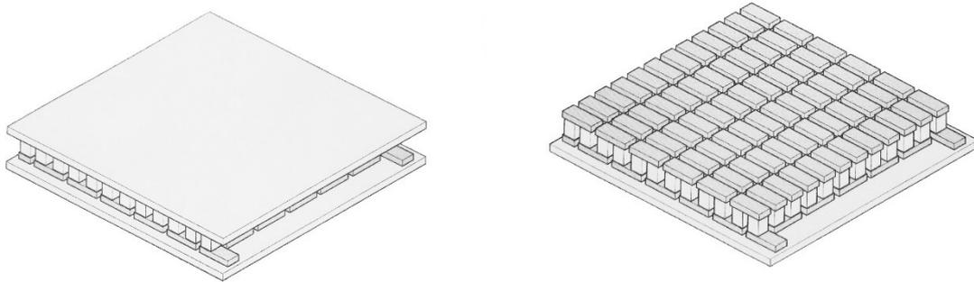
Figure 2: Schematic illustration of thermoelectric modules
