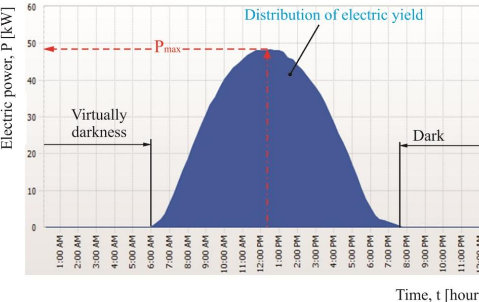
Figure 9: Power data on the 9<sup>th</sup> of April, 2021 in kW
