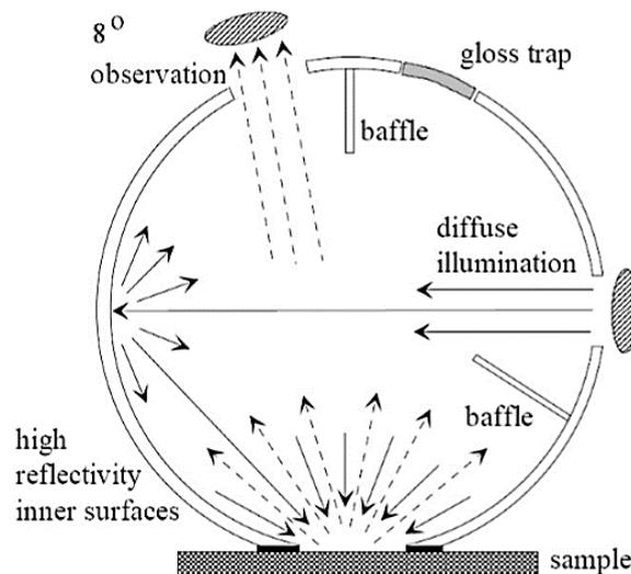
Figure 5: Measurement geometry  $de:8^\circ$
