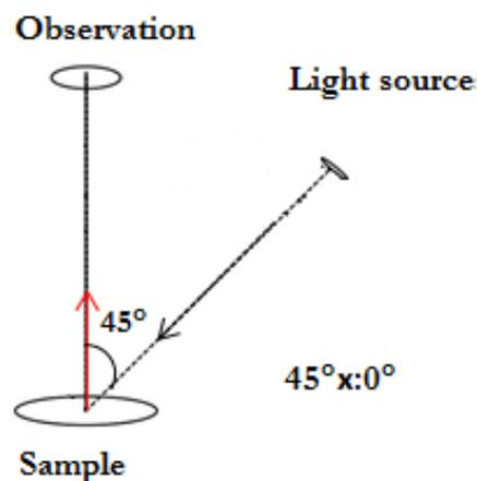
Figure 1: Directional geometry  $45^\circ x:0^\circ$
