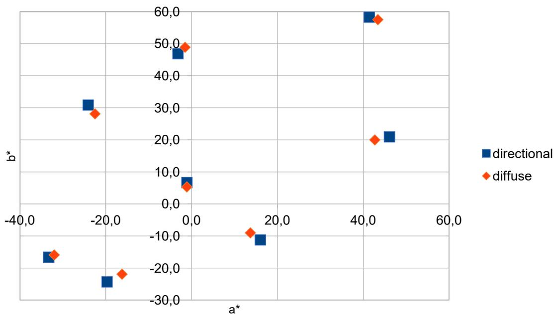
Figure 12: CIELAB  $a^*$ ,  $b^*$  values of the eight color samples with texture #1 on the chromaticity plane, obtained by instrument with directional (blue squares) and diffuse (orange diamonds) measurement geometry
