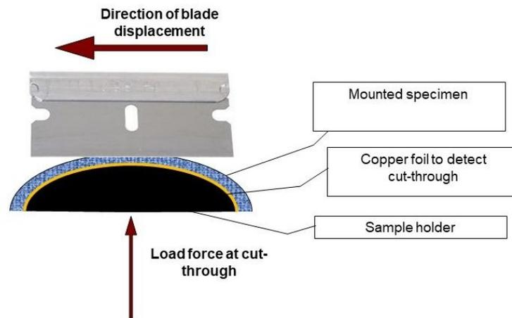
Figure 1: Schematic drawing of the TDM test method [3]
