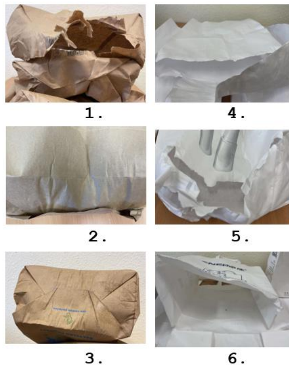
Figure 5: Visual inspection after moisture effect and load capacity testing
