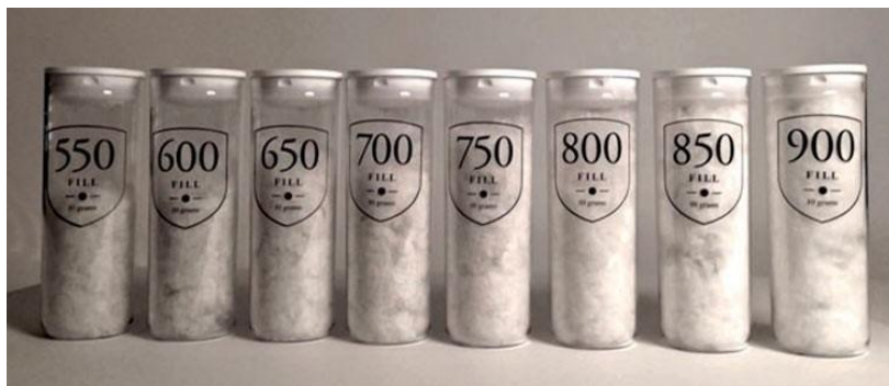
Figure 4: Fill power measuring tubes
