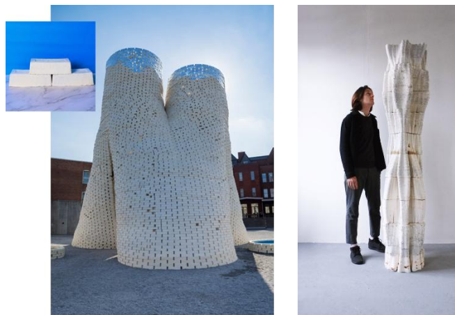
Figure 1: From left to right: 1) Ecovative's Grown.bio building bricks [16]; 2) The Living Studio: Hy-Fi Tower, led by David Benjamin, built from Grown.bio building bricks [12]; 3) Op't Oog columns, 3D printed [19]
